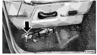
Jack Wing Bolt Remove the jack and tools by removing the wing bolt and sliding the assembly from under the seat.
